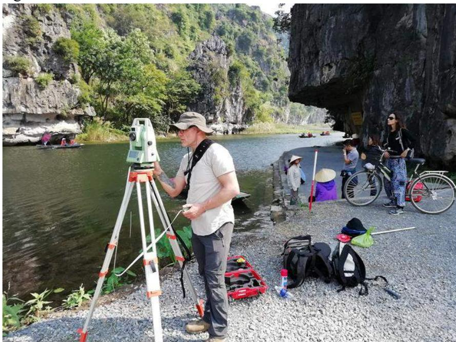
**Figure 2. Notch survey at Thanh Warf, Thai Vy using a Leica TS06 total station**
